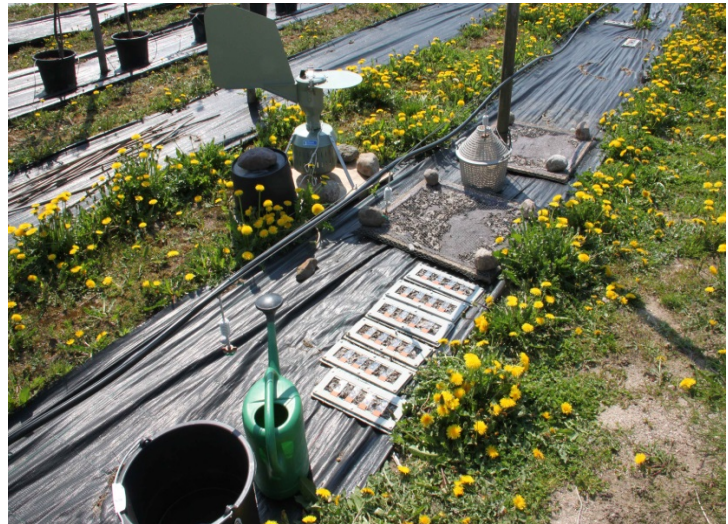
Figure 4: Equipment for measuring discharge of ascospores in relation to irrigation with different sizes of drops. Two spore traps are used: Slideholders and a Burkard volumetric spore trap.
