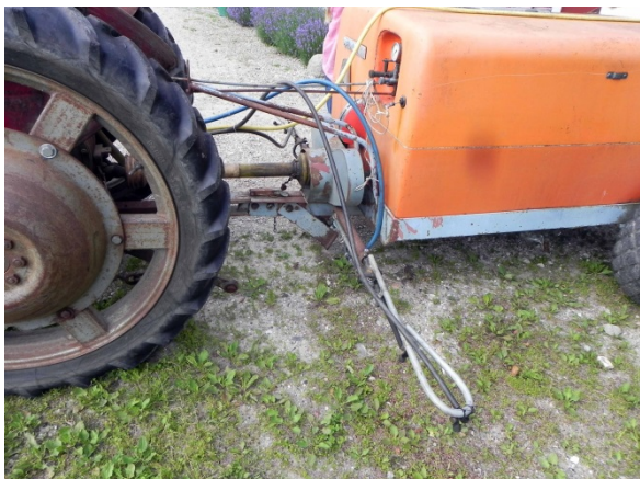
Figure 1: The waterwagon from the orchard Harndrup. It is a resused mistsprayer, where the pump was geared up. Mounted with a bar with sprinklers
