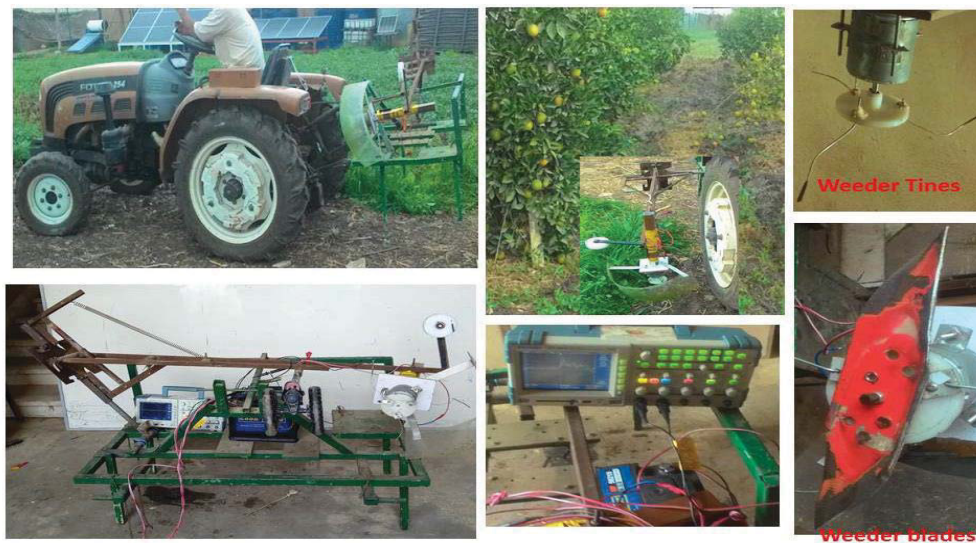
Figure 3: Display a manufacturing swing mechanical arm with electric Weeder in laboratory and field conditions.
