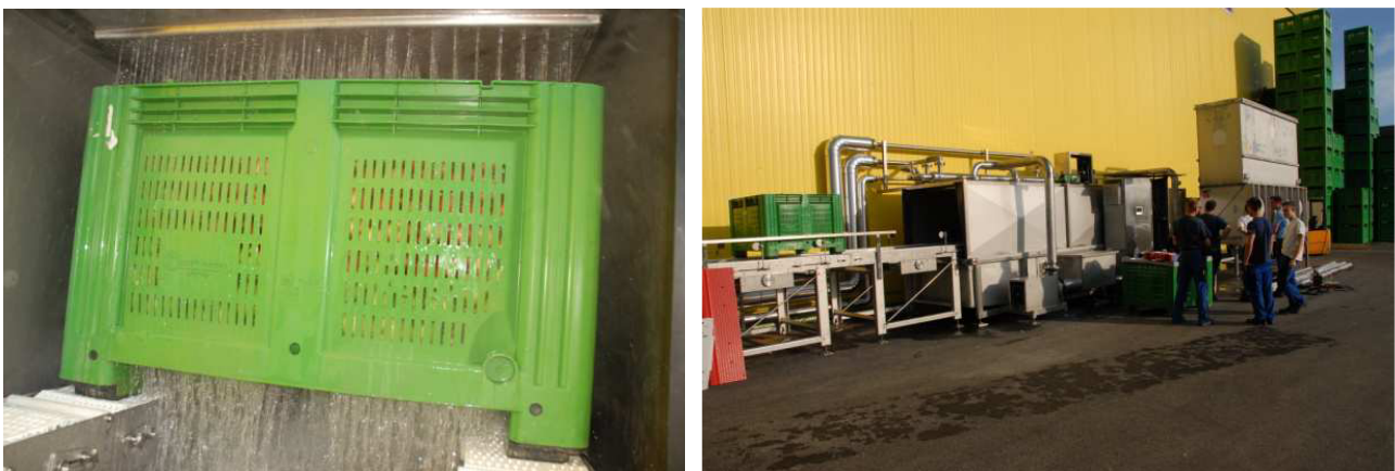
Figure 1: The process of the hot water shower (left); the hot water shower machine (right).
