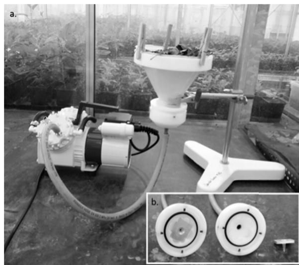
Figure 1: Design of an artificial ascospore release setup with a) the spore trap and vacuum pump and b) the mechanism of ascospore capturing.
