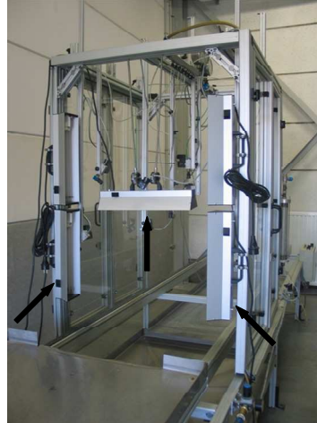
Figure 1: Representation of trial set-up with the motorised table. The black arrows indicate the position of the three different lights.
