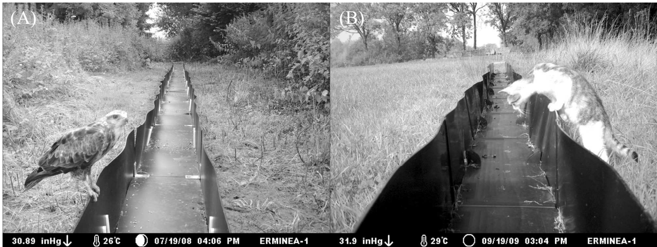
Figure 1: Experimental vole-trapping-fence consisting of HDPE panels (A) and prototype of a commercial modular trapping-fence (B) in practical field tests. The fences were frequently visited by buzzards (A) and domestic cats (B).
