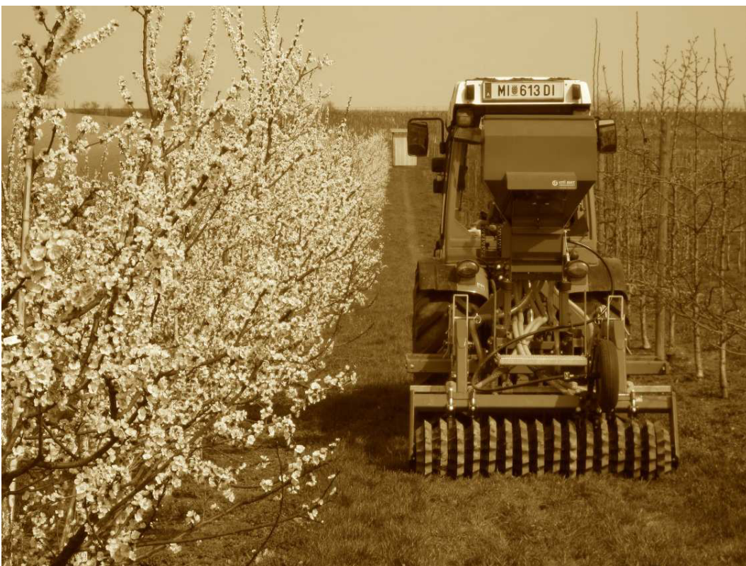
Figure 6: GreenManager® in flowering apricot orchard, cutting cover crop roots a few cm beneath the soil surface.
