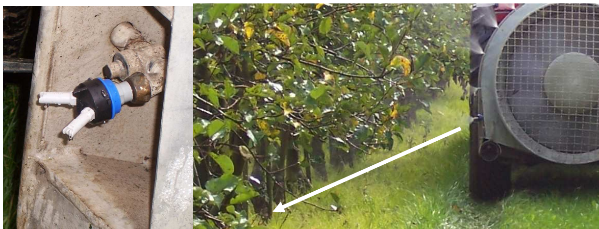
Figure 1: TWIN SPRAY CAP with nozzles and optimal direction of the twin cap towards the bottom part of the stem
