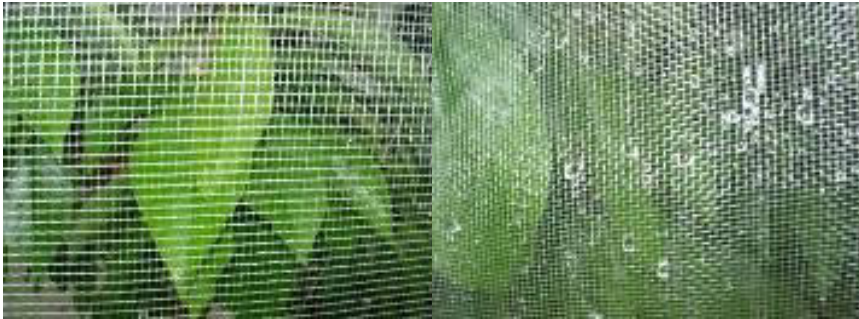
Figure 1: Overview of two different mesh sizes: medium 4x5 (left) / small 6x6 (right)
